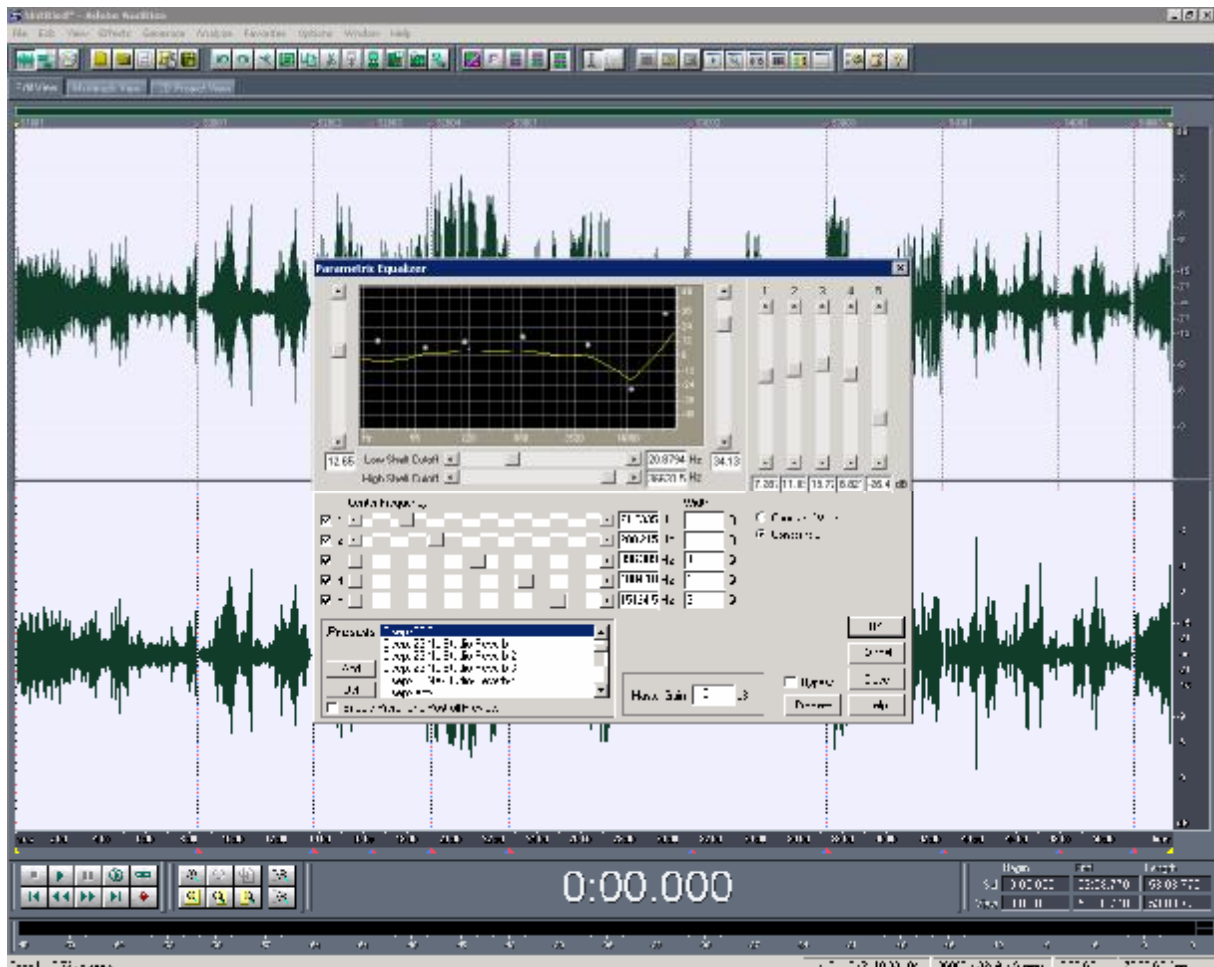
Figure 4: Equalizing with -15 dB output - mid section amplified
